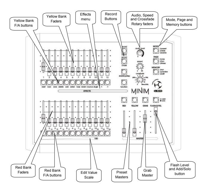
The front panel of the **MINIM** can de divided up into two areas:
